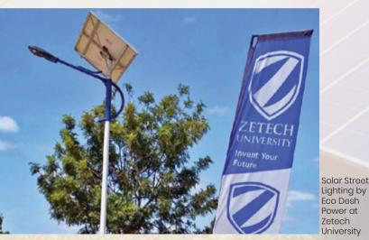
It is a comprehensive solution with state of the art components. We use polycrystalline solar modules giving 25 years warranty, LED light with over 2,500 lumen and 50,000 life cycles and high tolerance maintenance free batteries.
